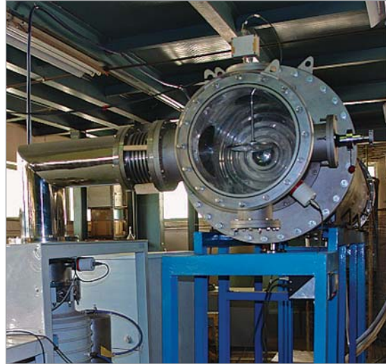
Fig.6: Front view of reflex triode with vacuum pumping system
