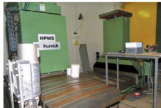
Fig. 5: Experimental arrangement for testing the detector with X-ray source
