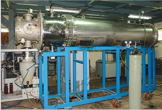
Fig. 5: Photograph of 1kJ Marx generator with reflex triode
